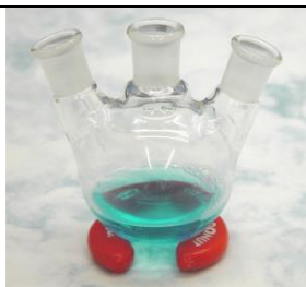
15 ml of solution in a 100 ml flask
