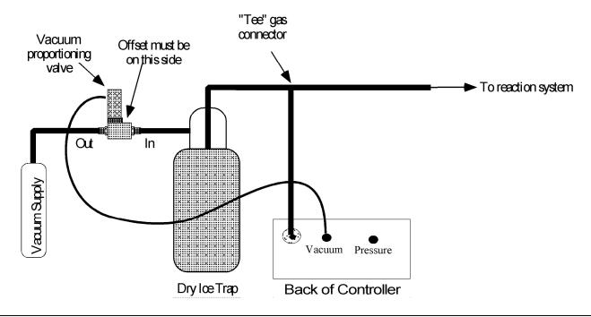
**NOTE:** The pressure proportioning valve is very sensitive to contaminates that cause the valve to stick. A high efficiency trap must be placed between the proportioning valve and the reaction system to protect the valve. Proportioning valves are not warranted against failure.
