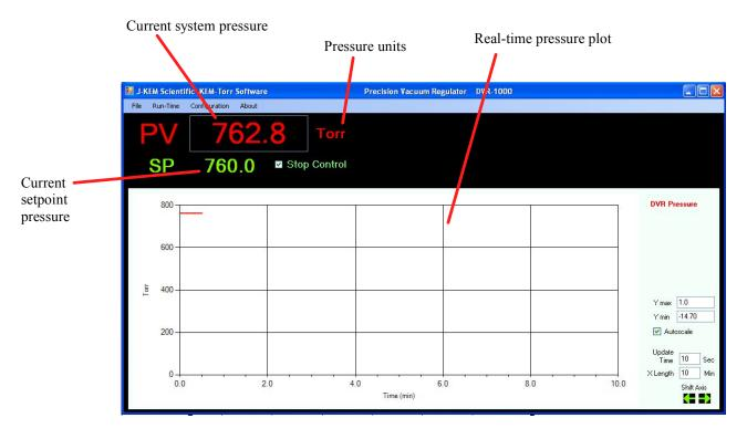
The software displays the sensed pressure and immediately begins to plot data. Note that pressures are displayed as 'Absolute' pressure.
