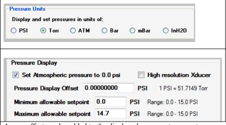
Specifies the default units for pressure display, data logging, and charting. After selecting the desired unit, the software must be exited and restarted for the change to take effect.
