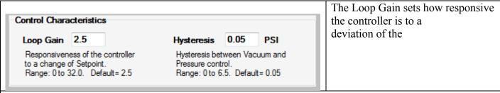
system pressure from the setpoint pressure. Low values product slow, but stable adjustments to bring the system pressure to the setpoint. High values result in a fast response to a deviation from setpoint, but can also result in unstable control. The default value is 2.5.
