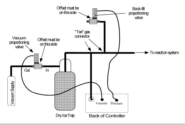
**NOTE:** The vacuum and atmosphere proportioning valves are very sensitive to contaminates which cause the valves to stick. A high efficiency trap must be placed between the vacuum proportioning valve and the reaction system to protect the valve. Proportioning valves are not warranted against failure.
