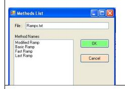
**Recalling a Ramp Program** – To load a saved ramp, select Recall Program form the Programs menu. A window appears that lists the names of the saved programs, click on the desired program, then click the OK button.
