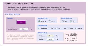
Now remove the vacuum source and allows the vacuum transducer to set at atmospheric pressure. Enter the current barometric pressure in the box titled "Actual Pressure" and click the Read button. Remember, pressures must be entered as Absolute pressure, so enter the actual barometric pressure, which is probably not 14.69 psi (i.e., exactly 1 atmosphere).
