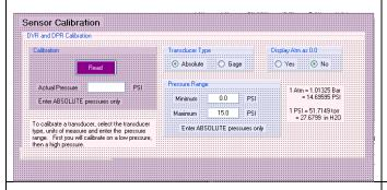
Click the calibration button to open the calibration input screen. Connect the vacuum transducer to a vacuum source and lower the pressure to any value below 0.01 psi. Enter the actual system pressure in the box titled "Actual Pressure" and then click the Read button.
