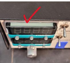
Turn on the controller and verify that all three buttons are operable.
