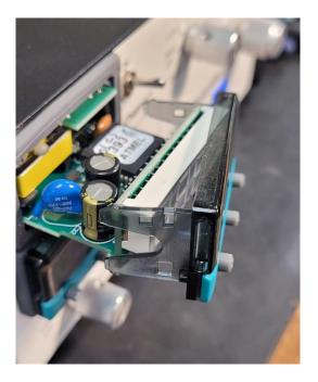
Align the new keypad with the front of the meter. Flex the sides of the keypad to allow it to slide into place.
