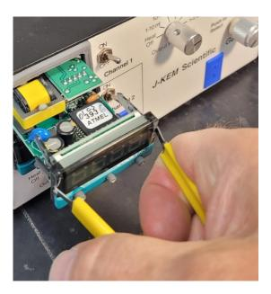
Gently pull the two tabs on each side on the keypad to release it from the meter.
