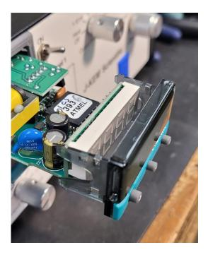
Ensure that the 2 holes on each side engage with the tabs on the meter.
