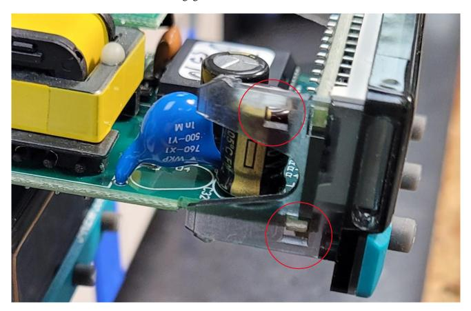
Firmly press the front of the meter until it rests against the rubber gasket.
