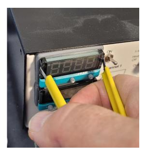
It is not necessary to remove the meter completely from the meter case. It is only necessary to pull it out far enough to access the sides of the keypad.
